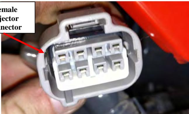
3) On the Ag Diesel Solutions module harness, the grey 8 pin male injector connector will connect to the female injector connector fixed on the engine. The Ag Diesel Solutions module harness can be routed along existing wire loom.
