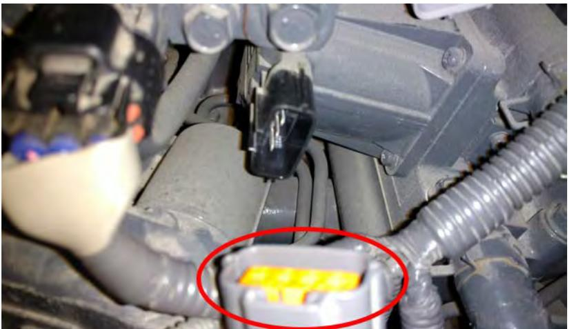
7) Plug the new male EGR Valve connector from the module harness into the stock female EGR Valve. Plug the Ag Diesel Solutions female EGR Valve connector from the harness into the stock male EGR Valve connector.
