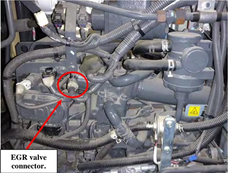
6) Unplug the stock EGR valve connector. Press and hold the release tab on the connector and gently pull the connector apart.
