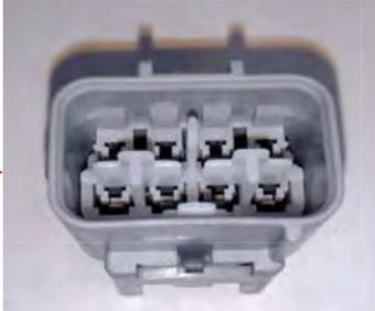
5) Locate the stock EGR valve connector. On a tractor, this connector is also accessible from the right hand side of the engine. This is a four pin connector that will be enclosed in a protective rubber weather seal.
